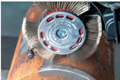
The bristle tips strike the surface, with kinetic energy, resulting in both corrosion removal and micro-indentation in the surface.
